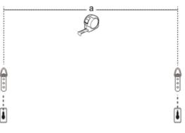
location. Mark two reference points (A, B) on the wall as shown. Make two insertion marks (C, D) centered along the line using the measurement "a
